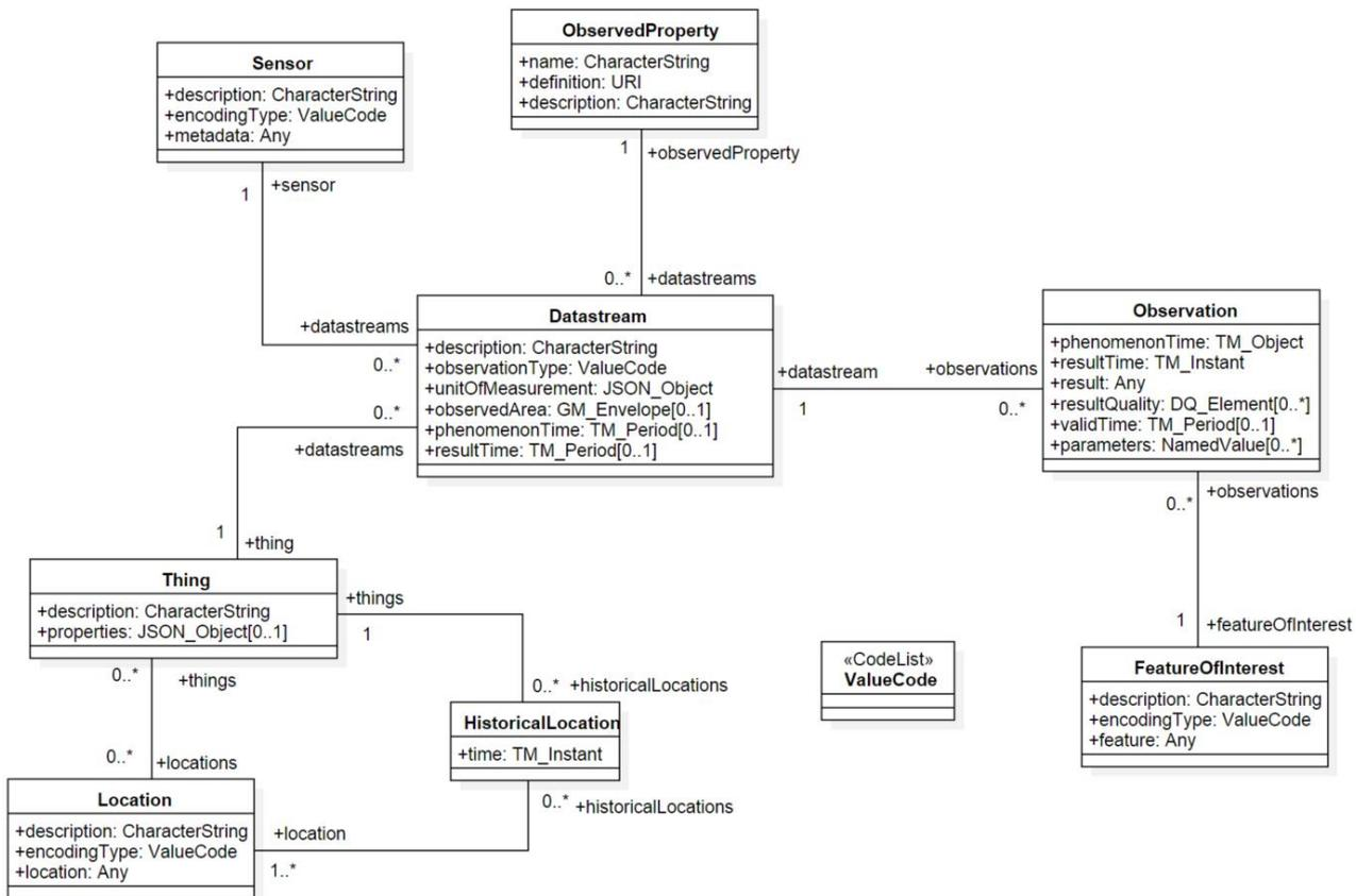
Figure 8: OGS SensorThings Static Model
