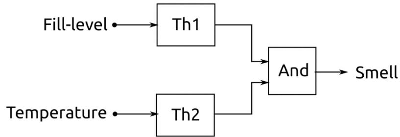
Figure 17. Bad smell detection query with event streams and threshold filters
