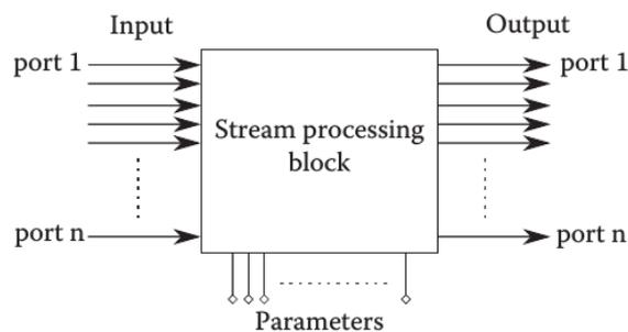
Figure 3. A generic stream processing block.
