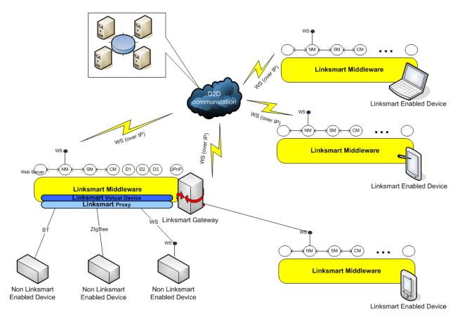
Figure 18: LinkSmart Example Device Network
