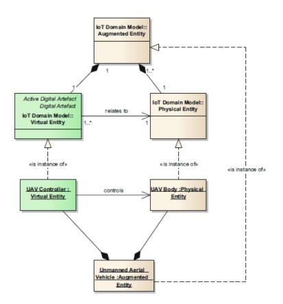
Figure 22: Example modelling using the Domain Model.
