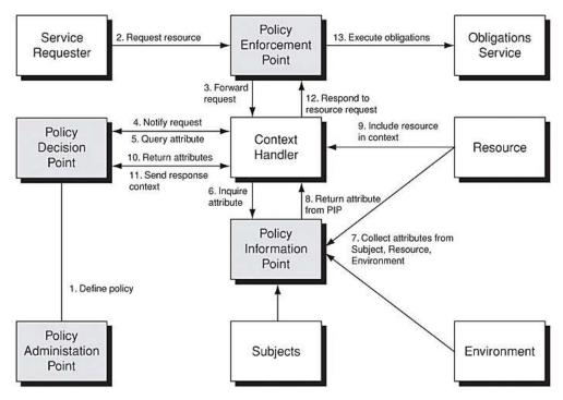
Figure 5: XACML Reference Architecture (Policy Enforcement Pattern)
