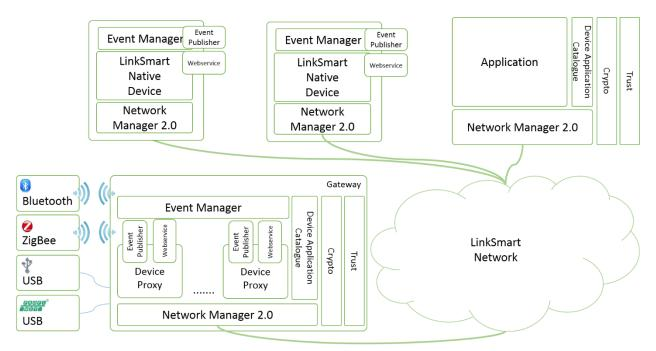
Figure 17: LinkSmart Example Concrete Deployment
