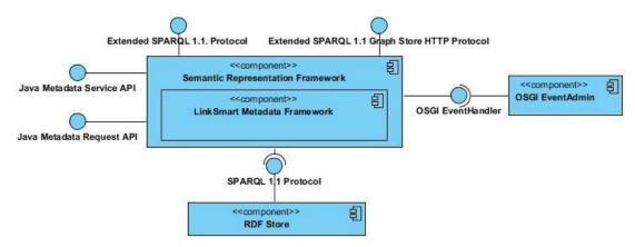
Figure 8: Semantic Representation Framework components and interfaces
