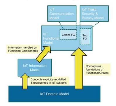
Figure 20: Sub-models of the IoT Reference Model (From (Bassi et al., 2013))
