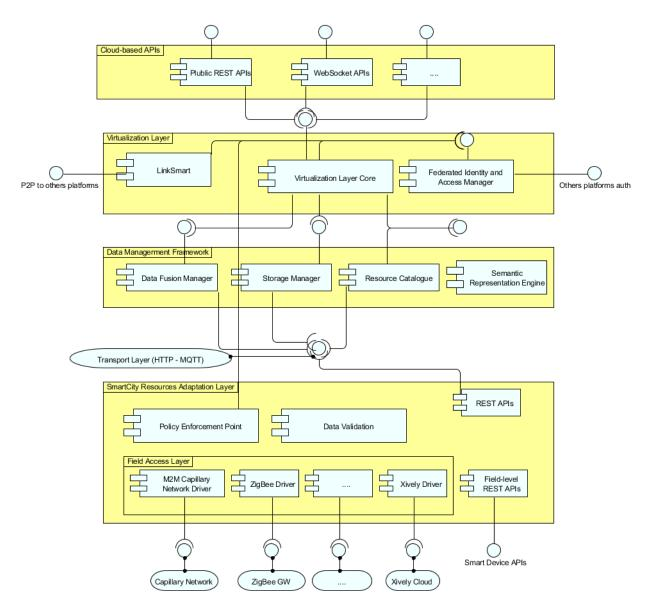
Figure 3: Component diagram of the ALMANAC platform
