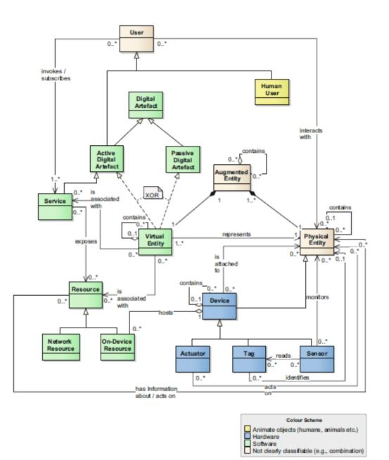
Figure 21: UML version of the IoT-A Domain Model
